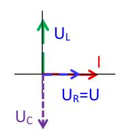
Note that at the resonant frequency, the voltages on terminals of inductor and capacitor are always equal but with different sign (phase lag 180<sup>o</sup>). Therefore the voltage on terminals of RLC dipole equals the voltage on resistor:
