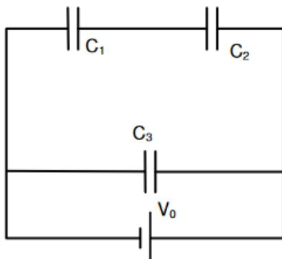
The circuit on picture is made up by two  $20 \mu\text{F}$  capacitors  $C_1$  and  $C_2$  connected in series and a  $100 \mu\text{F}$  capacitor  $C_3$  in parallel. The entire system is connected to a voltage source  $V_0=100 \text{ V}$ . Calculate:
